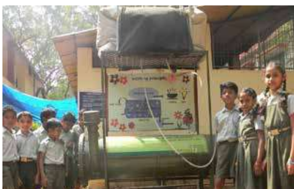
The food waste digester unit installed in Govt. UP school, Poojapura, TVM.
