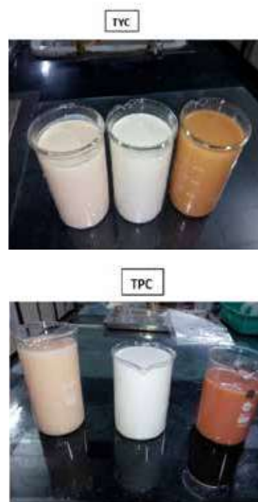
Feed Clay, non magnetic and magnetic fractions after magnetic separation in WHIMS
