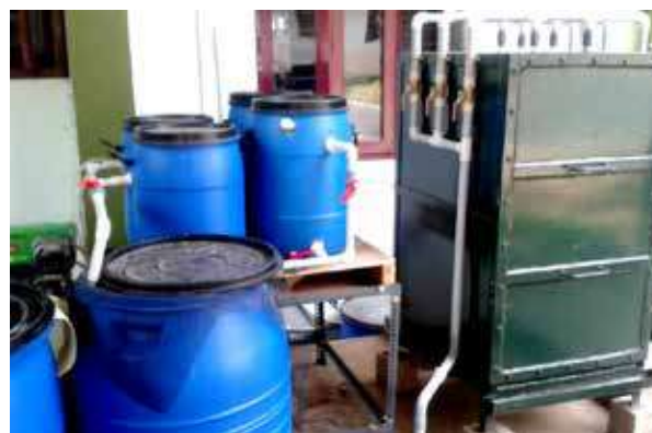
Demonstration scale soil treatment system
