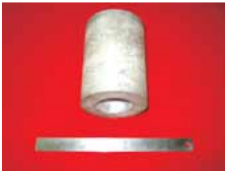
Centrifugally Cast LM13 Aluminium alloy Cylinder Liner
