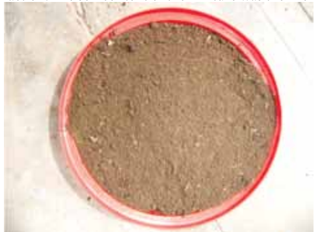
Photograph of compost produced from MSW through anaerobic leach bed treatment followed by aerobic composting
