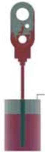
Simulated filling pattern of the cavity for a constant inlet pressure 1.12 atm.
