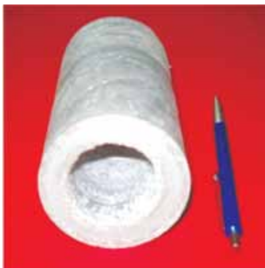
Cylinder casting fabricated by NIIST centrifugal casting machine
