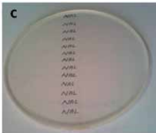
Solar cell cover with (A) Inorganic-organic hybrid coating (B) Hydrophobic nature of hybrid coating and (C) Photograph of NAL glass substrate coated with doped titania composition
