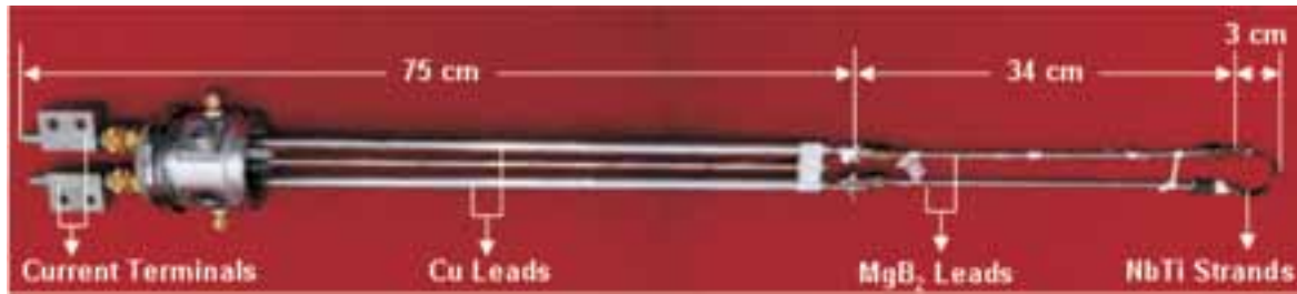
Vapor cooled superconducting current lead assembly
