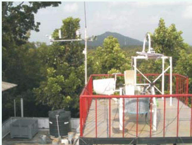
Experimental outdoor raceway pond reactor for algal growth studies
