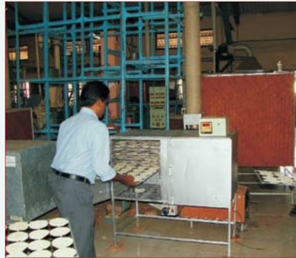
Redesigned (large) capacity Pappad drier; 14 trays, 280 Pappads/ batch
