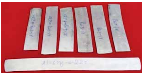
Fig.1 Rolled sheets (upto 2mm) of Al-Mg alloys containing Zr
