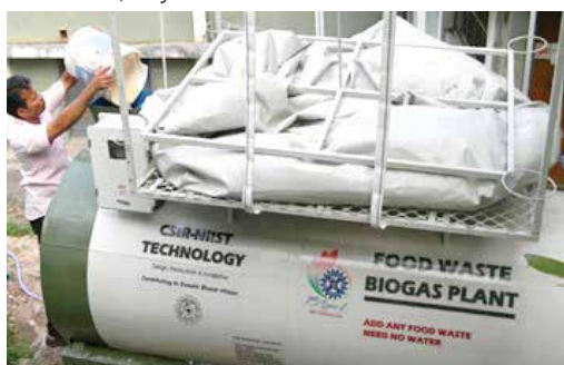
NIIST food waste biogas unit installed at RCC Trivandrum
